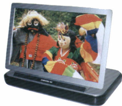
Figure 2: Samsung's 15.5 inch OLED monitor prototype is only 1.8 mm thick (81 Howard).
