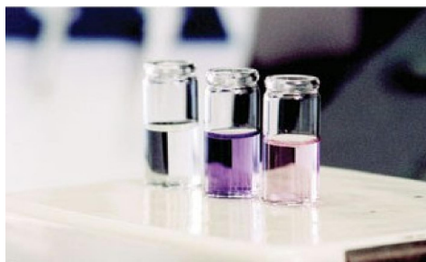
Figure 2: Demonstration of TAML activators with waste from paper mills. The container on the left is water, the container in the middle is water with waste and the last container on is the waste from a paper mill treated with TAML
