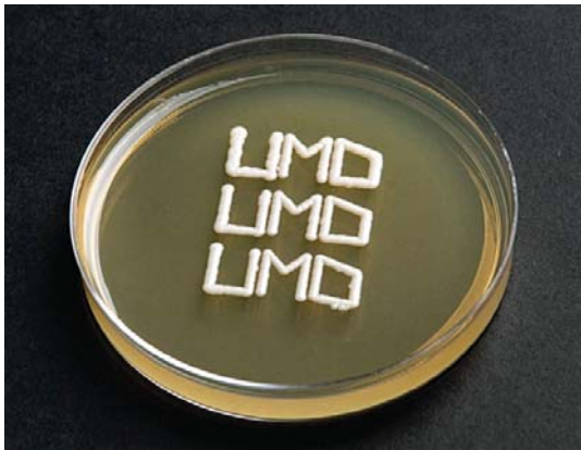
Figure 2. Printed Cells. Printed yeast cells are aligned to spell out “UMD” (University of Massachusetts Dartmouth), where they were created.
