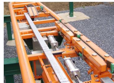
Brakes stop a steel roller coaster using friction.
