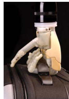
Figure 5. The power grip can be used to hold a mug or a briefcase.
