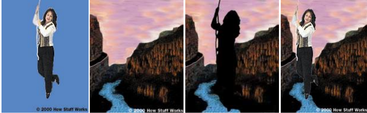
(From left to right) Figure 1- The foreground is shot in front of a blue screen. Figure 2- The background image is filmed in a separate location (or computer generated). Figure 3- A 'hole' is cut in the background image where the foreground image will be inserted. Figure 4- The blue screen is replaced by the background scene and the foreground scene 'fills in' the hole.
